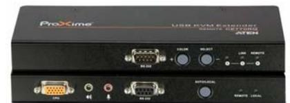
In addition, the CE770 features Deskew, an automatic delay line synchronizing function (ATEN patent) that corrects RGB color phase and timing errors that occur over long distance transmissions. It also enables you to manually tune the R/G/B signal settings.
