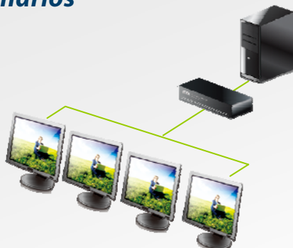
Duplicating a single source to multiple displays
