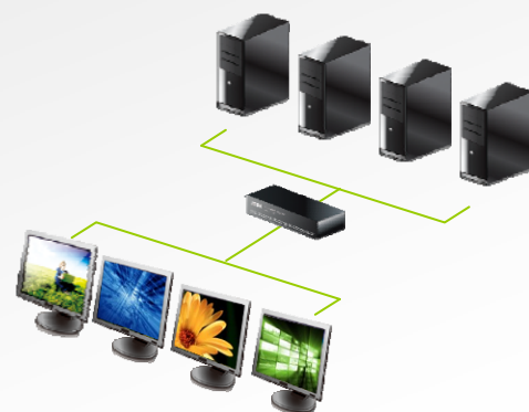
Routing multiple sources to many displays
