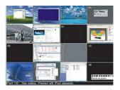
servers on screen as a panel array. Each server screen is periodically refreshed as well to let the administrator monitor the status on all servers. When the administrator moves the mouse cursor over the panel for one port, port details such as port name, connection status, access status and resolution are shown. If the administrator wishes to control one port directly, he simply clicks on the panel for that port to access the connected server.
