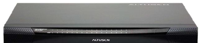
These models allow the use of both cascade (plugging server ports of one switch to the console ports of the next tier switch) and daisy-chain (plugging expansion ports into same-tier switch layer) architectures to
