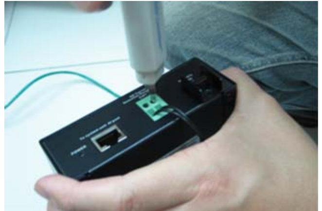
Once the sensor has been secured, use an UTP cable to connect the EA2210's RJ-45 port to the GN0116.
