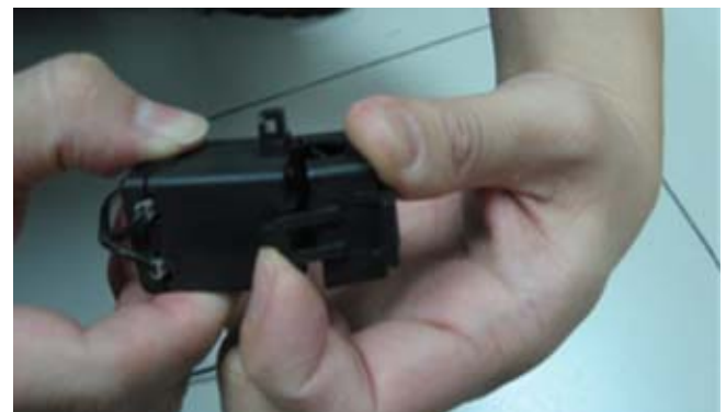
Place the power wire on the clip-on sensor device.
