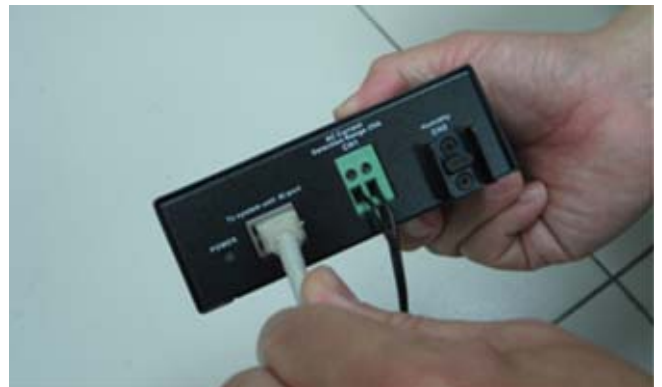
Use the Port 31/32 voltage-type Analog Input Port when connecting to the GN0116.
