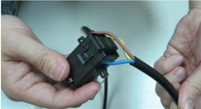
Connect the other end of the cable to the Terminal Block slot on the EA2110.
