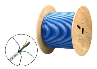
The 2L-2910 is a twisted pair cable engineered for optimum signal transmission at resolutions up to 4K including digital and <u>analogue</u> data, audio, and video applications. The cable supports sweep frequency up to 400 MHz and has been verified to meet performance requirements set by the <u>HDBaseT</u> Alliance.
