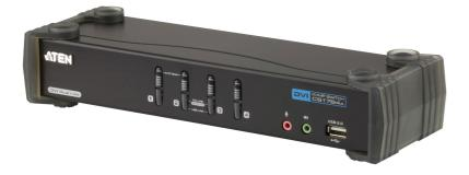
The CS1784A USB DVI Dual Link KVMP<sup>™</sup> Switch charts a revolutionary direction in KVM switch functionality. It combines the capabilities of a 4-port KVM switch with a 2-Port USB hub, while providing a DVI monitor interface and audio support. Moreover it carries advanced features, such as nVidia 3D Vision ready 120Hz 3D display support, gaming keyboard compatibility and port selection/switching using a mouse, aimed at giving you flexibility, convenience and enjoyment.
