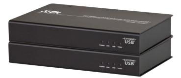
The CE610A USB DVI\_KVM Extender is a DVI and USB Extender that supports ExtremeUSB ® and HDBaseT technology. The CE610A can extend DVI and USB 2.0 signals up to 300 ft (100 m) from the source using a single Cat 5e/6 cable.
