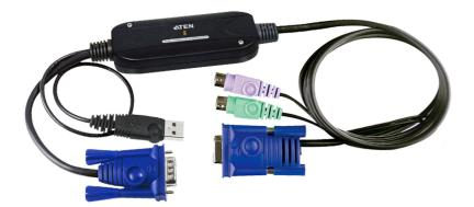
CV131B is a signal converter specifically designed for SUN systems. They can be used with KVM switches. Both models are easy to install and can be configured via the hotkeys on the keyboard.
