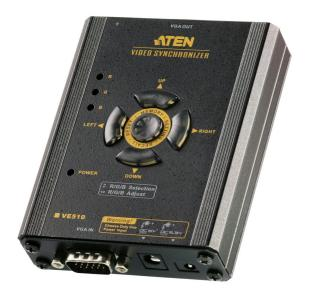
The VE510 <u>Video Synchronizer</u> is designed to compensate for video signal delays over large distances. The VE510's line synchronizing function corrects color phase and timing errors that occur over long distance transmissions. It also enables you to manually tune the R/G/B signal settings, store the settings and retrieve them later using the memory button.
