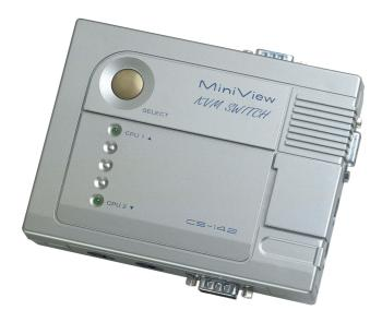
CS-142 is a KVM Switch with built-in PS/2. It can control 2 servers via a single console and allows users to switch between computers via the buttons on the upper side of the switch or the hotkey configuration on the console keyboard. It is the simplest and most convenient solution for multi-computer management.
