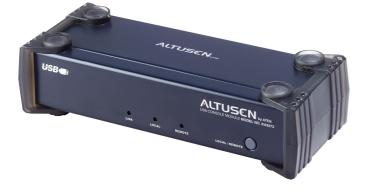
ALTUSEN KA9272 has one USB console which controls a local computer and the remote Martix KVM Switch 20060416233445004.jpg
