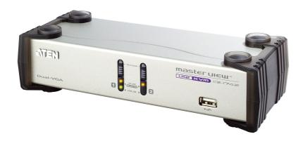
CS1742 2 Port KVM Switch integrates functions of video signal dual output and USB KVM switches. It allows a computer with dual-screen support to pair with two VGA/SVGA/Multisync displays via a USB keyboard and mouse. Furthermore, CS1742 provides 2 USB ports, allowing each server to share any USB peripheral device that is connected to this HUB.
