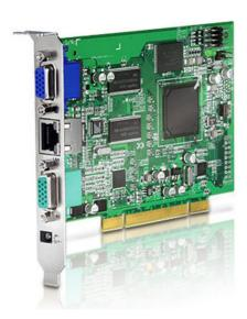
The IP8000 is a PCI card implementation of a control unit that provides "over-IP" access and control of the server it is installed in. The IP8000 allows multi-platform access and control of the server from remote locations using a standard Internet browser or with stand-alone Windows and Java applications
