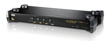
CS9134 is a KVM Switch with built-in PS/2. It can control 4 servers via a single console and allows users to switch between computers via the buttons on the front panel of the switch or the hotkey configuration on the console keyboard. It is the simplest and most convenient most convenient solution for multi-computer management. Moreover, it supports 3-tier connection via cascade. With 21 sets of CS9134, users can control 64 computers.
