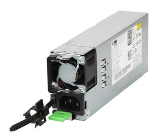
The VM3200 can be equipped with dual power modules to ensure that the system is always working. The power modules are hot-pluggable and can be easily replaced without shutting down the system. The VM3200 has two power slots that can connect to two different power supplies. If the primary power fails, the secondary power supply will automatically take over. ATEN ensures that your investment is well protected while delivering outstanding performance.
