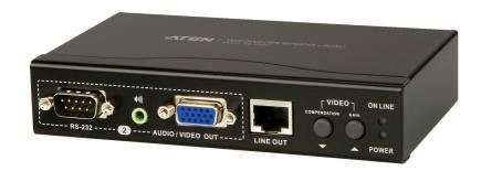
The VB552 VGA Over Cat 5 Repeater +Audio is an audio/video signal extension device which is compatible with ATEN Cat 5 Audio/Video splitters. The VB552 extends the audio/video transmission range an extra 500 feet (150m) over Cat 5e (or higher) cables. The use of an additional repeater means the audio/video signals can be transmitted over even longer distances, up to 1470 feet (450m).
