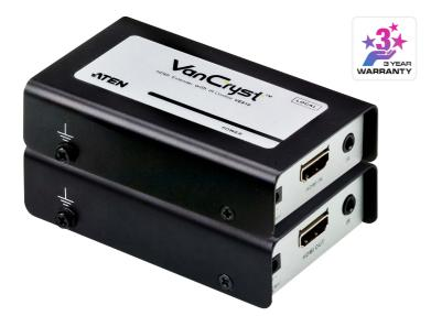
The VE810 HDMI Extender extends your HDMI display up to 198 ft (60 m) from your HDMI source device using two Cat 5e cables. In addition, VE810 is equipped with IR signaling pass-through which allows the IR channel to control from the remote to local unit, to control the HDMI source, or from the local to remote unit, to control the display device.
