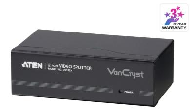
The VS132A Video Splitter is a boosting device that duplicates a video signal from one source to 2 output devices. Cascadable to three levels, the VS132A provides up to 8 video signals, in addition to extending transmission distance up to 98.5 feet (30 m), making it excellent for public broadcast systems.
