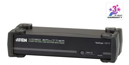
The VS172 2-Port DVI Dual Link Splitter with Audio combines DVI quality video and audio, taking signals from an audio/video source and replicating them to two audio/video outputs. This video splitter uses dual link technology, which offers high bandwidth capacity for added transmission power and faster refresh rates, thereby providing better video quality of viewing resolutions up to 2560 x 1600.
