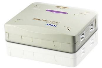
US401 allows 4 computers to share the same USB peripheral (e.g. printer, scanner and modem) under the foundation of one-at-a-time. Users can switch the computer controlling the peripheral from the reliable electronic button. There are LEDs indicating the status of the connection port.
