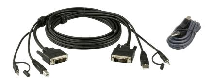
The 2L-7D02UDX2 Secure KVM Cable kit offers high- quality data connections between the Secure KVM Switch and your DVI servers and computers. The cable kit enables the connection of Video, USB Keyboard/Mouse/CAC, and Audio (Speaker), delivering excellent performance with ATEN PSS PP v3.0 Secure KVM Switches.
