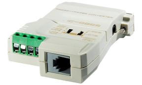
IC485S is a 2-way converter for converting RS-232 signals to and from RS-422/RS-485 signals in long-distance applications up to 1200 m (4000 ft.). It supports the connection of up to 32 hubs and features monitoring to confirm the data passing between devices.
