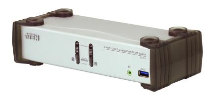
The ATEN CS1912 2-Port USB 3.0 DisplayPort KVMP<sup>TM</sup> Switch provides the latest innovations in desktop KVM switching technology to meet the increasing demand of higher video quality and file transfer rates on modern computers. The CS1912 provides superior resolutions up to 3840 x 2160 @ 30 Hz, a SuperSpeed USB 3.1 Gen 1 hub with 5 Gbps transfer rates and enhanced user-friendly operations.
