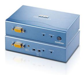
The CE252 allows access to your KVM installation through a local console, or a remote console placed up to a distance of 300m(1000') away. Both the local and remote units support PS/2 consoles. In addition to these features, the CE252 includes a convenient port at the remote unit to connect an extra computer. This allows the remote user to combine their desktop computer with the remote console for increase efficiency and productivity.
