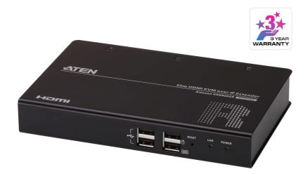
The KE8900SR Slim HDMI KVM over IP Extender is a compact and affordable high performance IP-based receiver that allows access to a computer system from a remote USB console (USB keyboard, USB mouse, HDMI monitor over an intranet, enabling users to locate computers in a secure and temperature controlled environment, which is isolated from users' workstation. All the extenders can be paired with any KE series\* receiver or transmitter for a savings solution that stays within budget.
