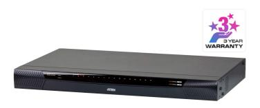
Aten's new generation of KVM over IP switches - KN series allows local console access and remote over IP access for operators to monitor and access their entire data center over a network using a web-based browser. In addition, they offer out-of-band access with external modern support for BIOS-level troubleshooting when the network is down.
