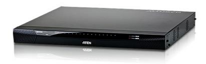
Aten's new generation of KVM over IP switches - KN series allows local console access and remote over IP access for operators to monitor and access their entire data center over a network using a web-based browser. In addition, they offer out-of-band access with external modem support for BIOS-level troubleshooting when the network is down.
