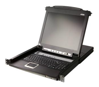
The CL5708 Slideaway – LCD KVM Switch series is a control unit that allows access to multiple computers from a single PS/2 or USB KVM (keyboard, video, and mouse) console. A single CL5708 can control up to 8 or 16 computers. As many as 31 additional KVM switches can be daisy-chained to the CL5708, so that up to 256 computers can all be controlled from a single KVM console.
