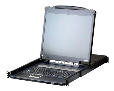
The CL5716I Slideaway™ LCD KVM Switch is a control unit that allows access to multiple computers from a single PS/2 or USB KVM (keyboard, video, and mouse) console. A single CL5716I can control up to 16 computers. As many as 15 additional KVM switches can be daisychained to the CL5716I, so that up to 256 computers can all be controlled from a single KVM console.
