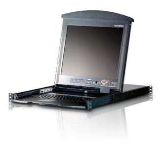
We understand that space in your data center is limited. That's why we've created the KL3116 LCD KVM Switch, a keyboard, video, and mouse (KVM) switch that offers secure access to 16 attached computers and mounts in only 1U of rack space. It features independently retractable 17" LCD monitor and keyboard with built-in touchpad. To maximize space in your data center the keyboard hides away when not in use, while the thin profile LCD monitor provides continuous monitoring of computers.
