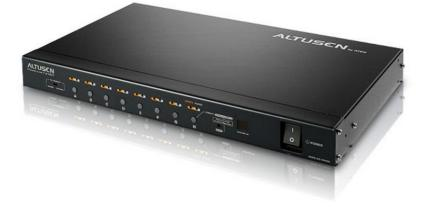
Altusen's PN0108 is equipped with eight hotpluggable ports for easy server room management. Each port can be individually controlled so that users can set the power on sequence and delay time for each port to allow equipment to be turned on in the proper order. On/Off scheduling allows for preset start/shutdowns/restarts on a daily, weekly,monthly basis. The PN0108 is the most convenient, reliable and cost effective way to obtain access to your server room remotely.\*
