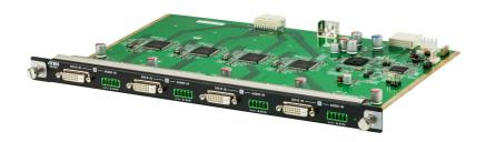
The VM7604 4-Port DVI Input Board is offers an easy way to route any of 4 audio/video sources to any of 4 displays, when used in combination with ATEN's Modular Matrix Switch.
