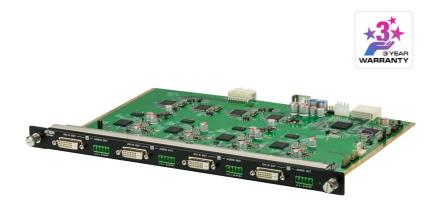
The VM8604 4-Port DVI Output Board is offers an easy way to route any of 4 audio/video sources to any of 4 displays, when used in combination with ATEN's Modular Matrix Switch.
