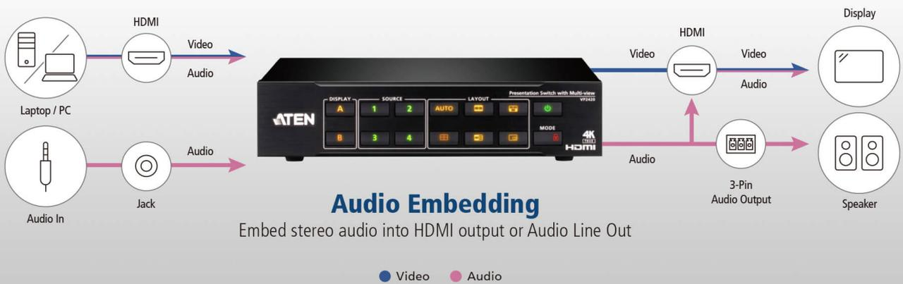
Managing presentations with the VP2420 is effortless, offering a wide range of control options such as front panel, push buttons, IR controllers, web GUI, [mobile app](#), RS-232, and Ethernet. Integration with control systems further enhances control, providing a comprehensive and streamlined presentation experience.
