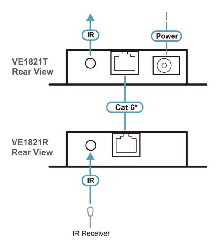
Note: Make sure to only connect VE1821T with VE1821R using models or third-party receivers may cause physical dama
