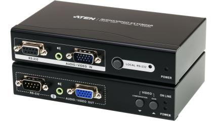
The VE200 Audio/Video Extender System allows you to extend the distance between the computer system unit and the display monitor by up to 200m/500ft for video resolutions of 1280x1024 @ 60Hz. It accomplishes this by means of a local transmitting unit (VE200L), and a remote receiving unit (VE200R), connected by Cat 5e twisted pair cable.
