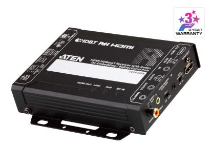
Featuring powerful Class A HDBaseT technology, the VE2812PR is a receiver for 4K HDMI video, audio, and control signals over a distance of up to 100 m via a Cat 5e / 6 / 6a or ATEN 2L-29330 Cat 6 cable. HDMI signal transmission extends further up to 150 m @ 1080p when the HDBaseT Long Reach Mode is enabled.
