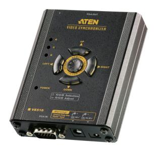
The VE510 Video Synchronizer is designed to compensate for video signal delays over large distances. The VE510's line synchronizing function corrects color phase and timing errors that occur over long distance transmissions. It also enables you to manually tune the R/G/B signal settings, store the settings and retrieve them later using the memory button.
