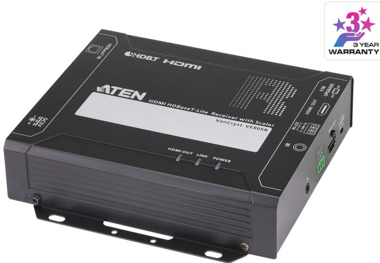
The VE805R HDMI HDBaseT-Lite Receiver with Scaler can be combined with ATEN HDMI HDBaseT products to extend a HDMI display up to 60 m from the HDMI source device using a single Cat 5e/6 cable or up to 70 m via a Cat 6a cable.
