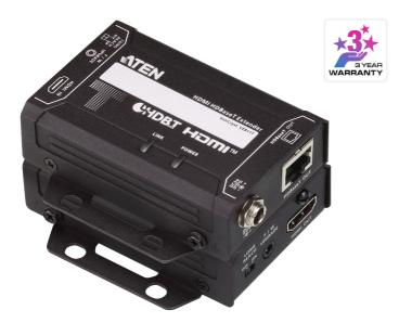
The ATEN VE811 HDMI HDBaseT Extender guarantees the optimum 4K HDMI signal transmission across up to100 m via a single Cat 5e/6/6a or ATEN 2L-2910 Cat 6 cable. In addition, with the support for Long Reach Mode, it extends HDMI signals @ 1080p up to 150 m via a single Cat 56/6 cable. The VE811 meets HDMI specification features including 3D, Deep Color, HD lossless audio formats and CEC pass-through. Plus, it supports Dolby Digital 7.1 ch and DTS HD audio.
