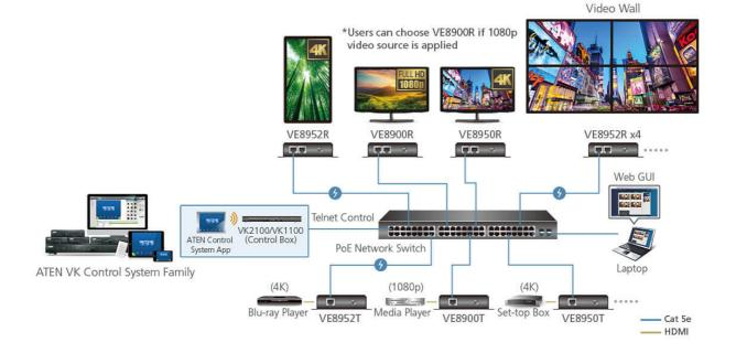
\*Note: VE8952 supports PoE and can be installed in combination with PoE network switches to reduce power cabling and additional power outlets. Before choosing the Network switch and installation, please refer to the Implementation Guide
