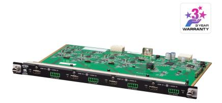
The VM7824 is a True 4K HDMI input board that works with an ATEN Modular Matrix Switch to offer an easy way to route 4 HDMI audio/video sources to 4 displays with True 4K high-definition images support. In addition to the HDMI interface that carries digital A/V signal, the VM7824 also provides 4 stereo audio input ports that enable stereo audio embedding.
