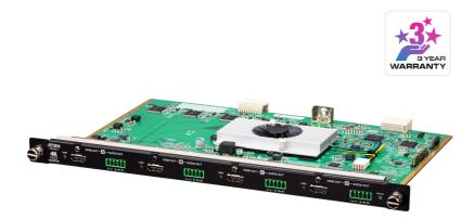
The VM8824 is a True 4K HDMI output board that works with an ATEN Modular Matrix Switch to offer an easy way to route 4 analog/digital audio/video sources to 4 HDMI displays with True 4K high-definition images support. In addition to the HDMI interface that carries digital A/V signal, the VM8824 also provides 4 stereo audio output ports that enable HDMI audio extraction.
