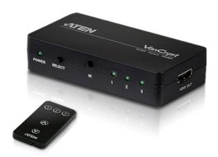
The VS381 3-Port HDMI Switch allows you to quickly and easily connect 3 HDMI input sources to your HDMI display device. It allows convenient switching between digital devices such as DVD players, satellite receivers and digital camcorders. You can select the desired input source via a remote control unit or pushbuttons located on the front of the switch.
