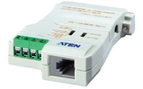
IC485SN is a 2-way converter for converting RS-232 signals to and from RS-422/RS-485 signals in long-distance applications up to 1200 m (4000 ft.) – without the need of an external power supply.
