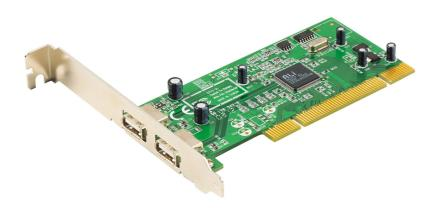
IC220U is a PCI card with 2 USB ports. It supports hot plug and PnP.
