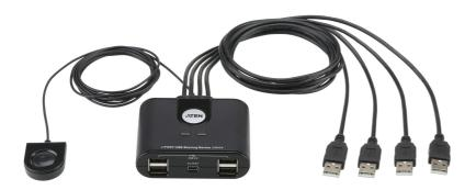
The US424 is a 4-port USB peripheral sharing device that enables 4 computers to share the use of 4 USB devices – a keyboard, mouse and up to two peripheral devices. It eliminates the added expense of having a separate USB keyboard, mouse and peripheral device(s) for each computer. The US424 all-in-one design allows for a neat and tidy installation – no need to connect 4 separate USB cables to the computer, thus eliminating cable clutter.
