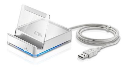
The CS533 Tap is a control unit that allows access to one computer and two Bluetooth devices from a USB keyboard and mouse. The CS533 Tap converts normal USB keyboard and mouse signals into Bluetooth connections to allow for easy sharing between your computer and bluetooth devices.
