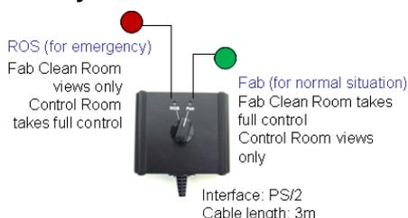
ATEN provides the customized firmware to work with Priority Control Box. The solution is used to assign the control priority between Fab cleaning room and control room.
